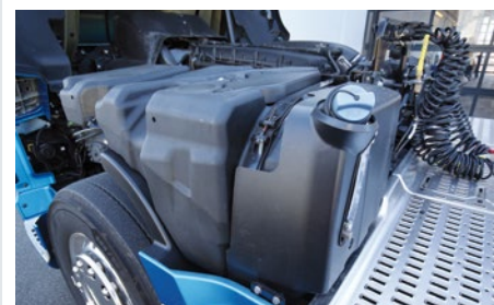
DAF installs the AdBlue tank in a raised position
